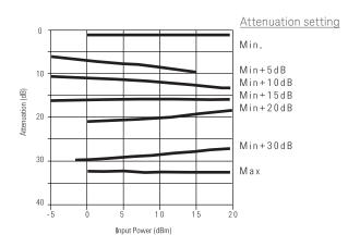
Figure 8. Attenuation vs. input power @ 2.0 GHz1
