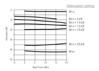
Figure 9. Attenuation vs. input power @  $10.0~\text{GHz}^1$
