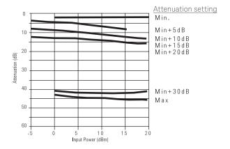
Figure 12. Attenuation vs. input power @ 22.0  $\mathrm{GHz^1}$
