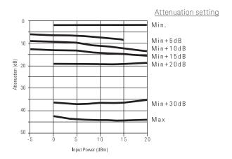
Figure 10. Attenuation vs. input power @ 14.0 GHz<sup>1</sup>
