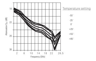
Figure 19. Attenuation vs. temperature @ 30 dB attenuation<sup>1</sup>
