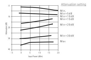
Figure 7. Attenuation vs. input power @ 50.0 MHz<sup>1</sup>
