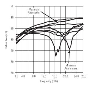
Figure 6. Output return loss vs. frequency<sup>1</sup>
