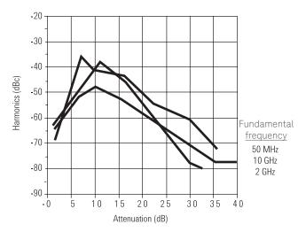
Figure 13. Second harmonic suppression vs. attenuation, input power =  $0.0~\mathrm{dBm^1}$
