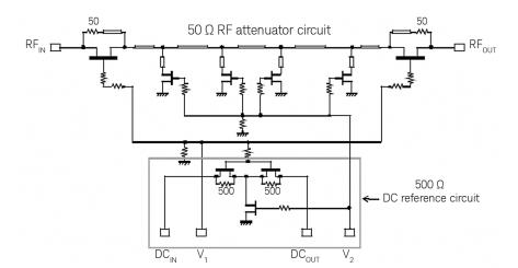
Figure 1. Schematic
