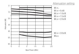
Figure 11. Attenuation vs. input power @  $18.0~\text{GHz}^1$
