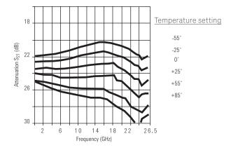
Figure 18. Attenuation vs. temperature @ 20 dB attenuation<sup>1</sup>
