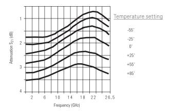
Figure 17. Attenuation vs. temperature @ 10 dB attenuation¹
