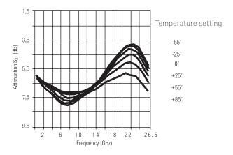
Figure 16. Attenuation vs. temperature @ 5 dB attenuation<sup>1</sup>
