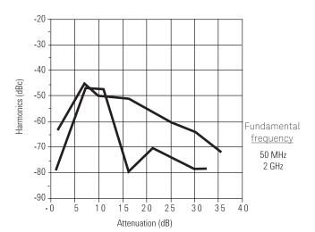
Figure 14. Third harmonic suppression vs. attenuation, input power =  $0.0~\mathrm{dBm^1}$
