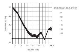
Figure 20. Attenuation vs. temperature @ maximum attenuation<sup>1</sup>
