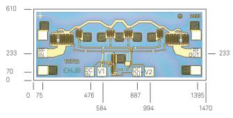
Figure 2. Bonding pad locations
