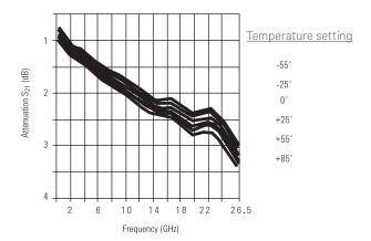
Figure 15. Attenuation vs. temperature @ minimum attenuation<sup>1</sup>
